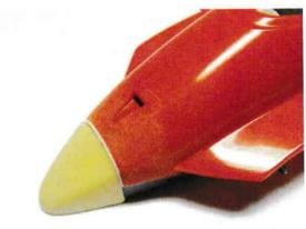
Check alignment between bodywork and resin nose
