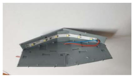
9. Wire the stripes and install the power supply.
