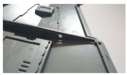
4. Drill a hole into part C5 for the tower power supply.
