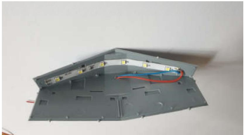
9. Wire the stripes and install the power supply.
