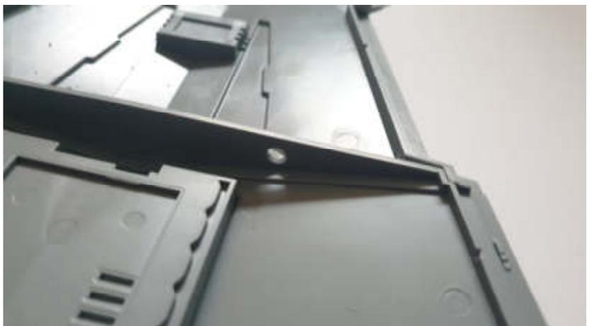
4. Drill a hole into part C5 for the tower power supply.
