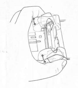
To turn the both front wheels, move the wheels by holding on both tires with your fingers as shown in the Figure.
