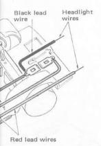
connecting the lead wires to the nals of the battery box, bend the nals down.
