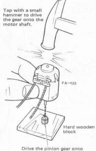
Drive the pinion gear onto the motor shaft until the outer surface of the gear is even with the end of the shaft.
