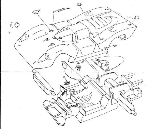
Note that the axles are offset so they may be mounted to adjust the wheelbase. The taillights load from inside the shell. Before any cementing, make sure to dry fit all parts and trim, if neccessary. Great care is needed to trim out the headlamp cowls, so a set of plugs are provided for vac-forming additional parts.
